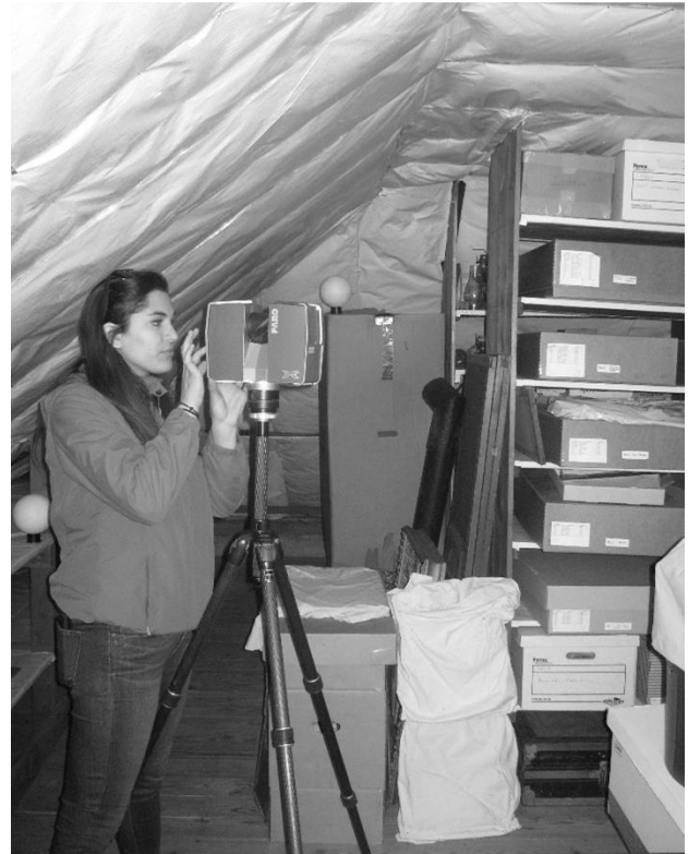
Melody Padrah setting up the scanner to survey the attic of the main building. Two of the magnetic orbs are visible on the shelf behind her and on the box in the background.
